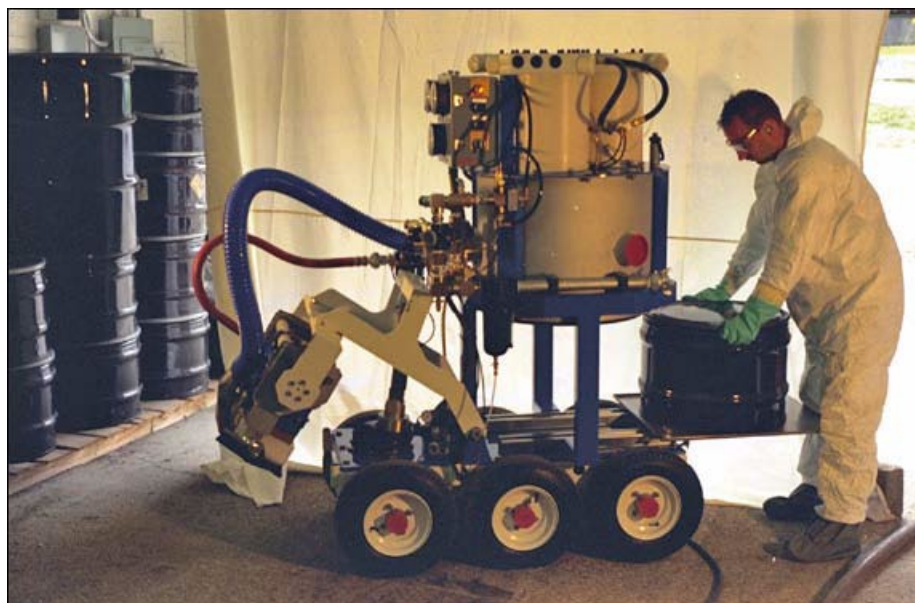
圖 1.2.11 PENTEK Moose® 遙控地板粗琢機[22]
