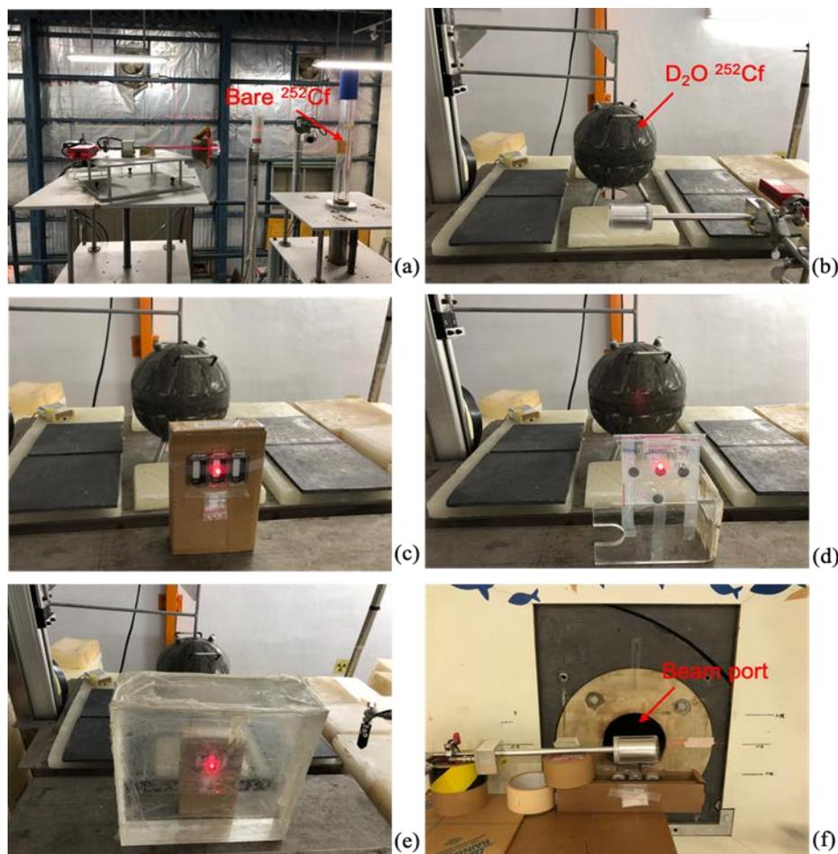
附圖 Irradiation experiment setup of OSLNs, TLDs and the TEPC in (a) bare <sup>252</sup>Cf field, (b) D<sub>2</sub>O moderated <sup>252</sup>Cf field, (c, d) D<sub>2</sub>O moderated <sup>252</sup>Cf field without compensator, (e) D<sub>2</sub>O moderated <sup>252</sup>Cf field with compensator, (f) NTHU-BNCT beam port.
