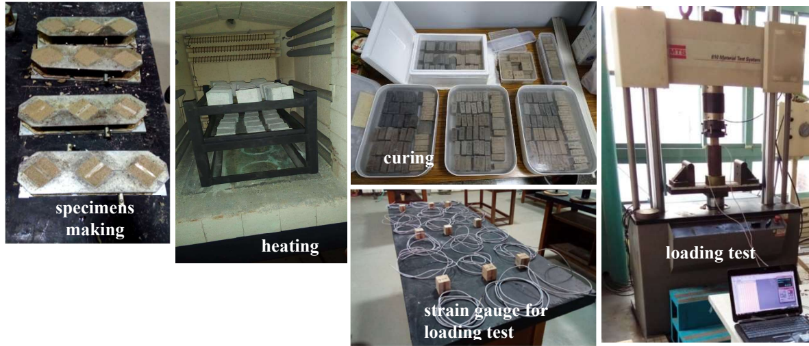
Fig. 2. Experiment design and specimen preparation for NLU
