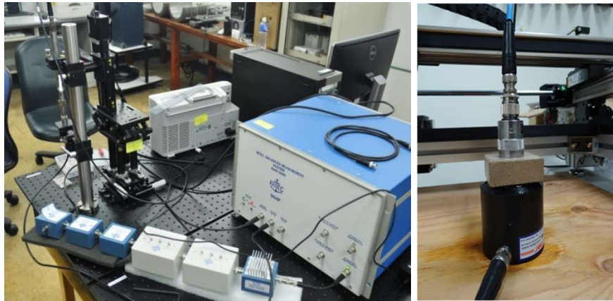
Fig. 1. The settlement of NLU technique for cement mortar specimen inspection
