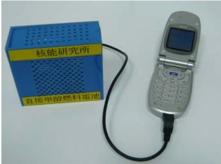
Small DMFC cell pack with MEA using home-made catalyst Pt/CNT and Pt-Ru-Ir/CNT
