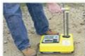
A moisture density gauge indicates whether a foundation is suitable for constructing a building or roadway.
