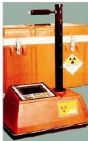
A moisture density gauge indicates whether a foundation is suitable for constructing a building or roadway.
