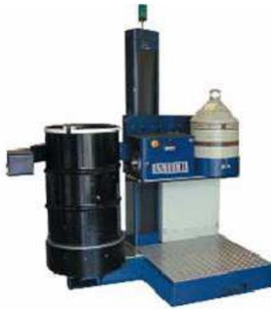
圖 5-4 Ortec SGS Segmented Gamma Scanner
