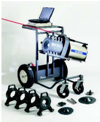
The ISOCS Detector, Cart, and Shield Component s
