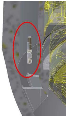
Picture 5: Sampling device at RPV wall close to the calotte
