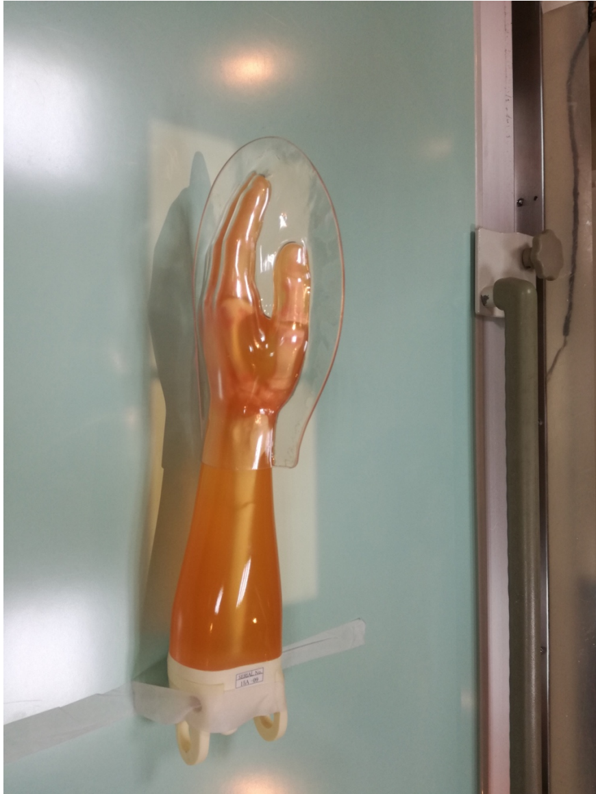
Figure 13: Experiment setup and Kyoto Kagaku hand phantom (Optional part of PH-2/2B).
