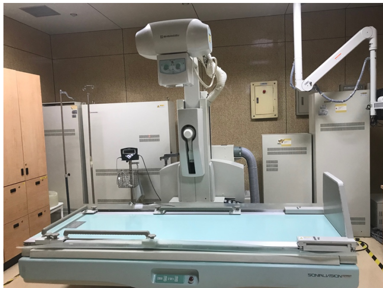
Figure 3: Shimadzu X-ray digital X-ray digital radiography, fluoroscopy, and tomosynthesis.
