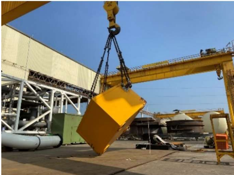
Figure 27: A safety test of an INER-LRW-C2 low-level radioactive waste container at the INER
