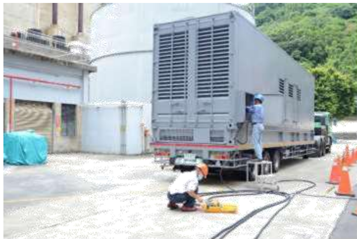
Figure 42: A power connecting drill by using a 4.16kV power supply vehicle at Chinshan NPP in 2021
