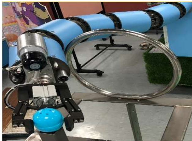
Figure 28: A test on the turning function of the serpentine robotic arm's obstacle avoidance at the INER
