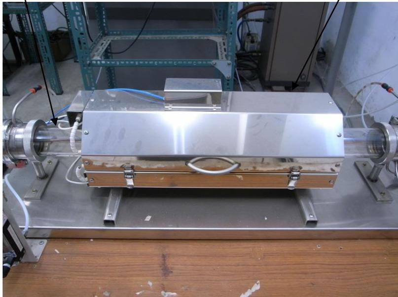
Fig. 5 Photograph of the environmental furnace for aging treatment.
