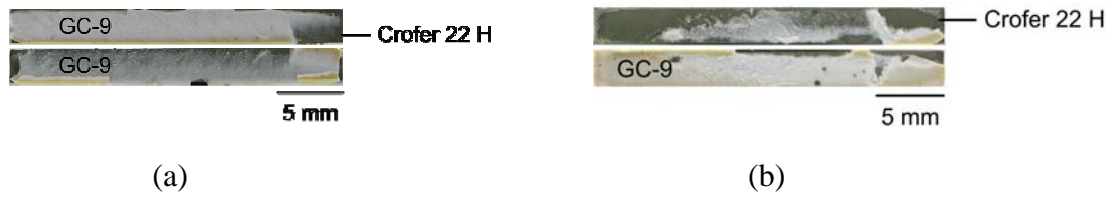
Fig. 32 Failure patterns of tensile specimens of POHT900S tested at (a) RT and (b) 800 °C.
