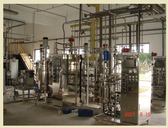
↑ Hydrolysis / Fermentation System for Cellulosic Bioethanol
