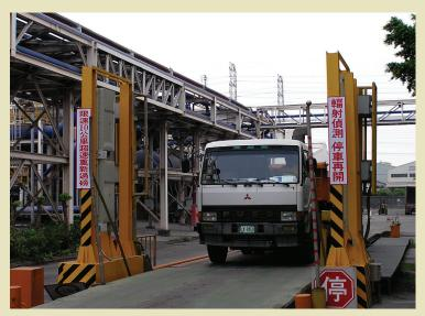
↑Portal type radiation detector in a steel mill
