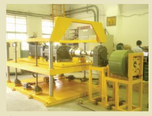
↑The 200kW Dynamo Test Station
