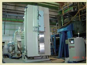
↑ Large Screw-rod Plasma Surface Modification System
