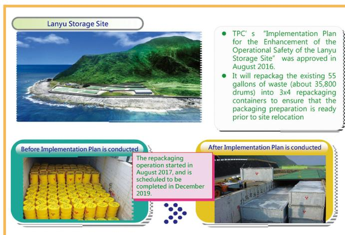
▲ Schematic diagram of the implementation plan for increasing the operation safety at the Lanyu Storage Site
