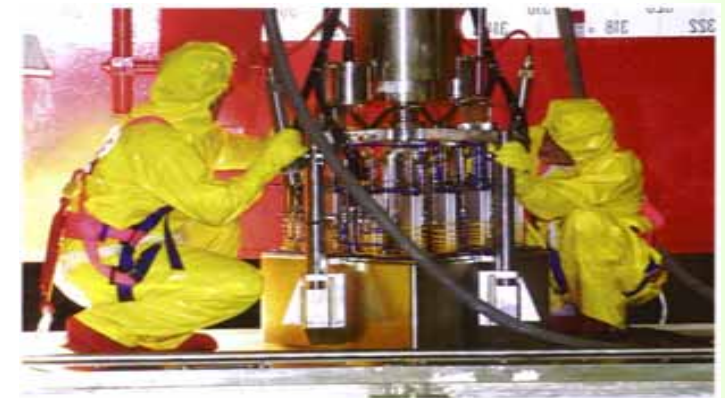
Sipping hood being disconnected from refueling platform mast after completion of sipping tests
