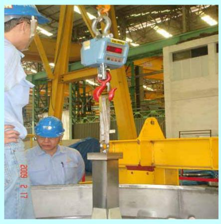
Dummy fuel plug in test during final acceptance check
