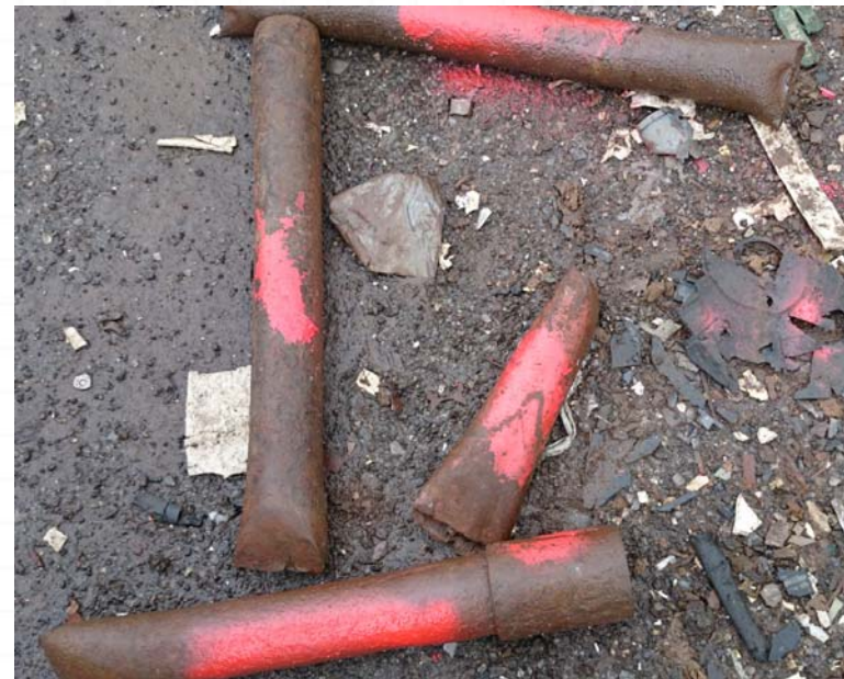
scale contaminated by NORM
