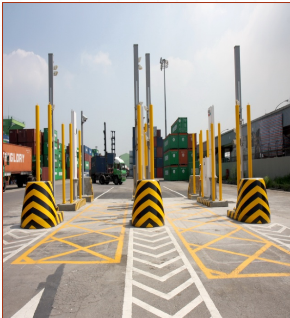
Radiation portal monitor as primary inspection
