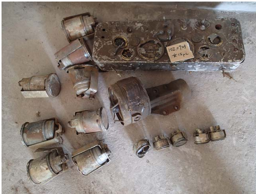
Gauges containing Ra-226
