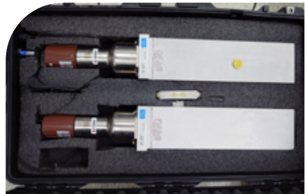
SPARCS for Aerial Radiation Detection with the Upgraded MCA Nuclear Instrument Module
