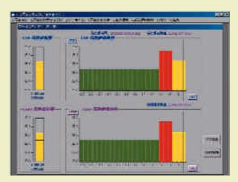
A TIRM-2 Risk Trend Graph for Core Damage Frequency (CDF) and Large Early Relief Frequency (LERF) Under Powered Operation
