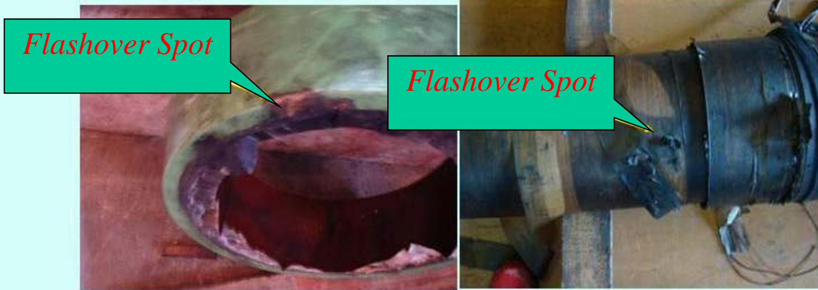
Flashover spot on capacitor paper layers
