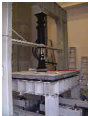
Use DPC sensor to detect the damage of broken reinforced concrete plate
