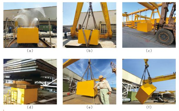
C2 容器試驗:(a)噴灑(b)吊掛(c)振動(d)堆積(e)正向墜落(f)傾角墜落 Tests on C2 container: (a) water spray (b) hanging (c) vibration (d) stacking (e) straight drop (f) angle drop
