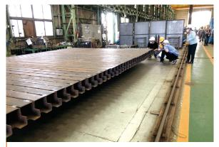
核二廠乾式貯存設施密封鋼筒燃料方管製程作業檢查 Taksforce Inspection for the square tube manufacturing process for the fuel in the dry storage facility's sealed drums in the Kuosheng NPP
