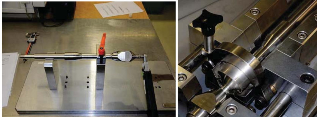
Figure 11. Fixtures used for mounting of WC UEP and staking (crimping).
