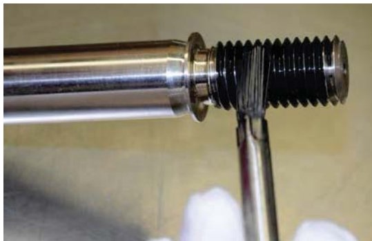
Figure 9. Typical application of [ ] thread lubricant.
