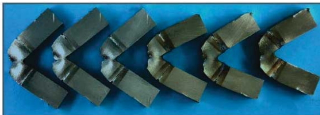
Figure 57. Charpy-V Impact Test Specimens after Testing.
