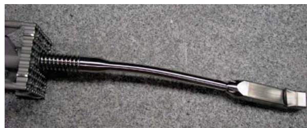
Figure 61. Connecting Bolt and WC after Testing.
