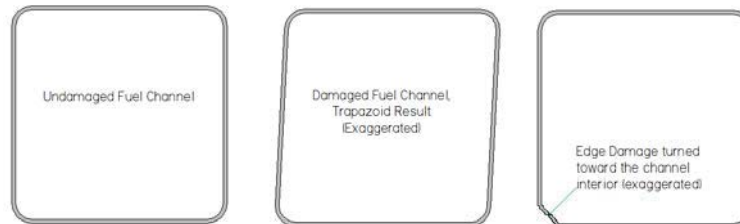
Figure 66. Possible Effects of FC Damage (exaggerated for understanding).
