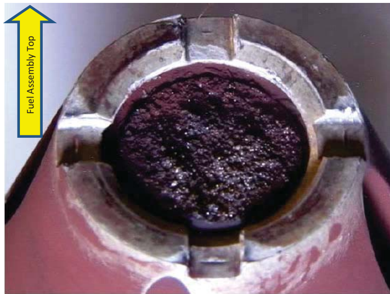
Figure 5. Lower receiving connection at the top of the central water channel.
