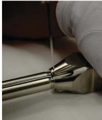
Figure 13. Inspection of finished connection using a feeler gauge.
