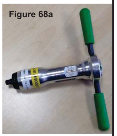
Figure 68. Click torque wrench with clutch release mechanism.
