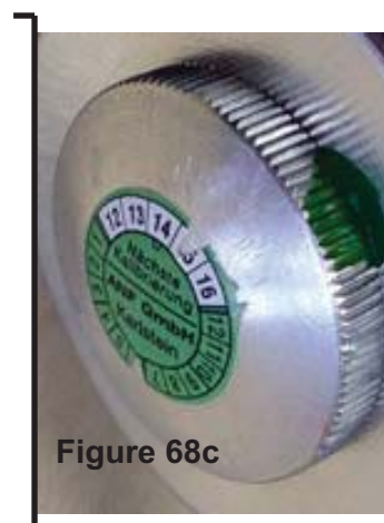
Figure 68. Click torque wrench with clutch release mechanism.
