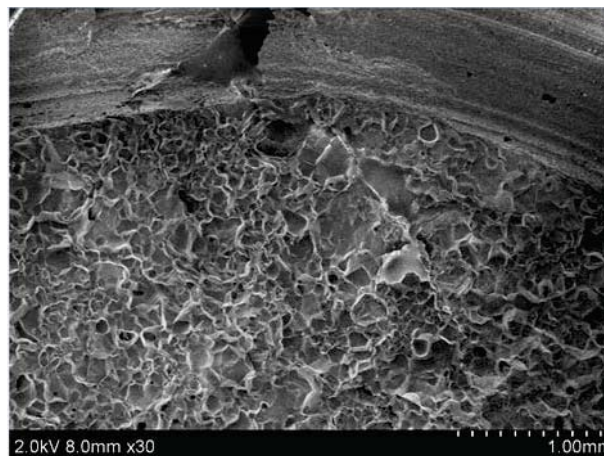
Figure 26. R1.1, 0° position, showing trace of small crack.
