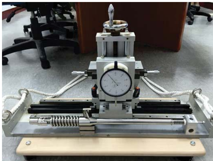
Figure 30. Straightness measurement setup.
